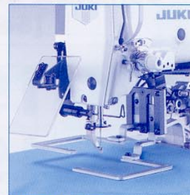
LK-1920SA (Pneumatic separately driven feeding frame)
