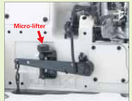
Bottom and top differential-feed micro adjustment mechanism
